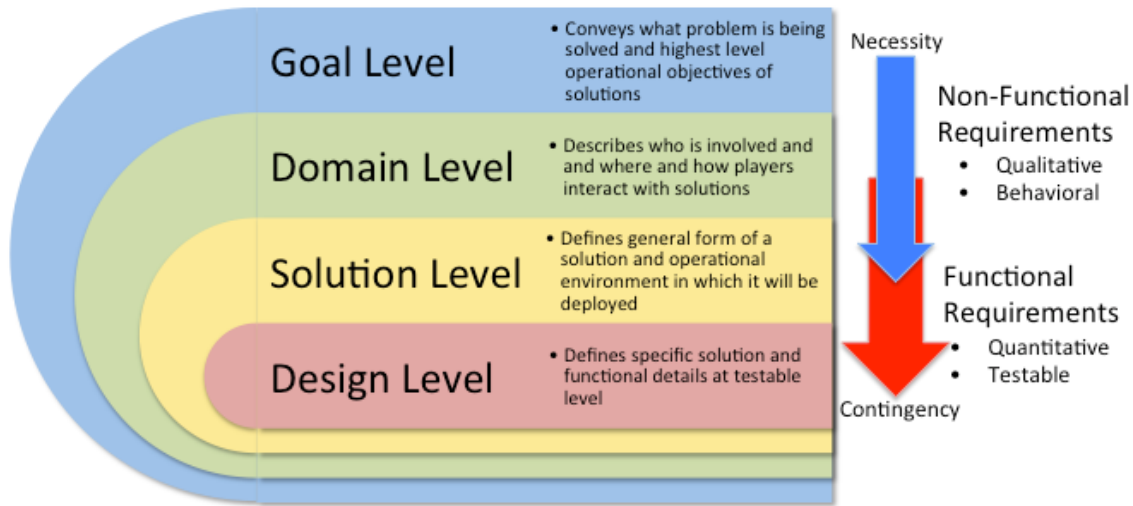
Figure 1.1. Levels of Increasing Specificity of Requirements
